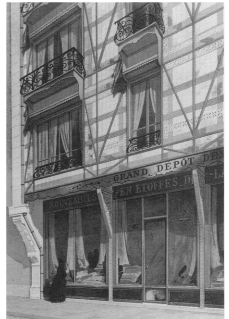
9. Viollet-le-Duc, street building with a modern iron frame and ceramic infill. ( Entrétiens sur l'architecture , atlas [Paris: A. Morel et Cie, 1864], plate 36.)
